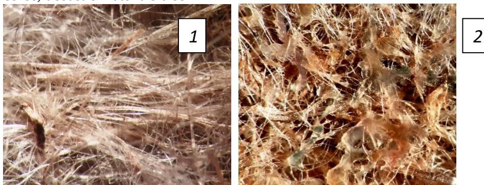
Fig. 1. Microphotographs of a sound-absorbing composite based on flax and polypropylene fibers: 1 – original fibrous canvas (thickness 10-12 mm); 2 – pressed panel (thickness 4-5 mm) [1]
