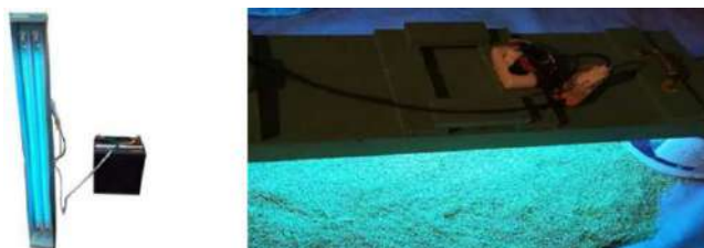
1-rasm. a) Sholi urug‘larini ultrabinafsha nurlantiruvchi laboratoriya stendi, b) Sholi urug‘lariganur berish jarayoni
