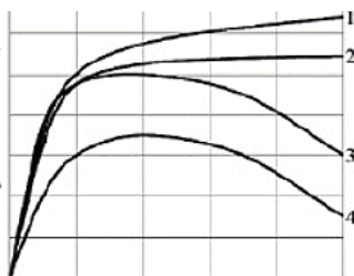
Figure. Concrete durability curves: 1 – in a humid environment; 2 - in an air environment, 3, 4 in a corrosive environment of varying intensity
