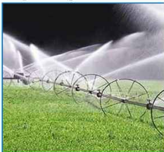
1.5-rasm. Yomg'irlatib sug'orish ko'rinishi
