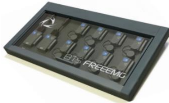
2.9-rasm. BTS FreeEMGning zaryadlash qurilmasi
