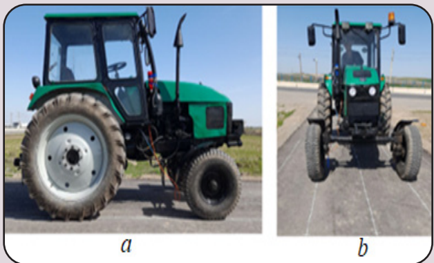
3-rasm. Tajribaviy traktorning minimal bazasida sinusoidal trayektoriya bo'ylab harakati
