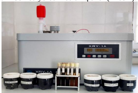
1-rasm. XRY-1A rusumli kalorimetrik bomba.
