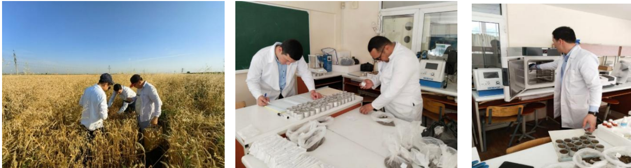
Figure 3. Field and laboratory workflow for determining soil moisture: weighing wet soil samples (left) and drying in MICROEST (right)
