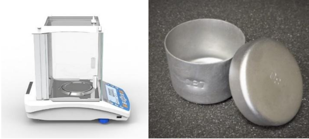
Figure 2. HERMES MAX 220 g electronic analytical balance and aluminum moisture tin used in soil sample preparation.
