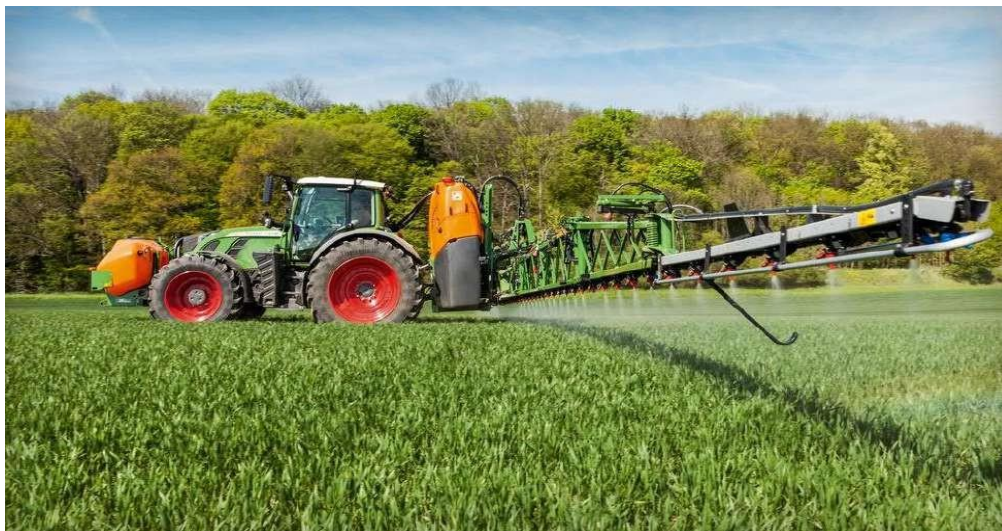
2-rasm. Shtangalik purkagichining texnologik kish jarayoni
